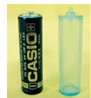
Photo 2 Left: Conventional battery Right: Methanol cartridge (PET bottle)
