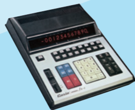
fx-1 1972: A scientific calculator that enabled one-key operation for a variety of calculations such as trigonometric and exponential functions.
