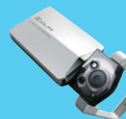
Green Slim Projector 2010: Thanks to a hybrid light source using both laser and LED technologies, this environmentally responsible projector offered high brightness without using a high-pressure mercury lamp. A light source lifespan of 20,000 hours was also achieved.
