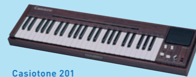
Casiotone 201 1980: An electronic musical instrument based on the concept of a keyboard that anyone can enjoy playing. It produced sounds that mimicked various types of acoustic instruments using a Consonant-Vowel System developed by focusing on temporal variations in sound.
