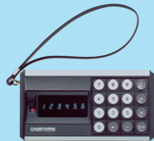
Casio Mini 1972: The world's first personal calculator. It sold for just 12,800 yen thanks to a simple component design, a single-chip LSI and a six-digit display. The Casio Mini became widely popular in ordinary homes, and the series sold a total of 10 million units. It also contributed to semiconductor development.
