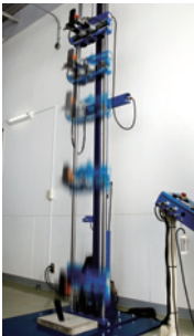
Handheld terminal: Drop test
