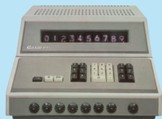
001 1965: The world's first electronic desktop calculator with a memory function.
