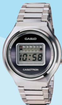
Casiotron 1974: This electronic watch was based on the concept of timekeeping by adding one second at a time. It was the world's first wristwatch to feature an automatic calendar that correctly adjusted the number of days for each month.
