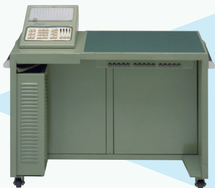
14-A 1957: The world's first compact all-electric calculator. It boasted quiet, high-speed calculation in a unit small enough to be used in an office. The 14-A offered reliability thanks to Casio's development of its own relays, which were dust-resistant and less prone to contact failure. It was adopted by many companies and research institutions, and reduced the labor required for office and technical computing.
