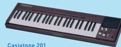
Casiotone 201 1980: An electronic musical instrument based on the concept of a keyboard that anyone can enjoy playing. It produced sounds that mimicked various types of acoustic instruments using a Consonant-Vowel System developed by focusing on temporal variations in sound.
