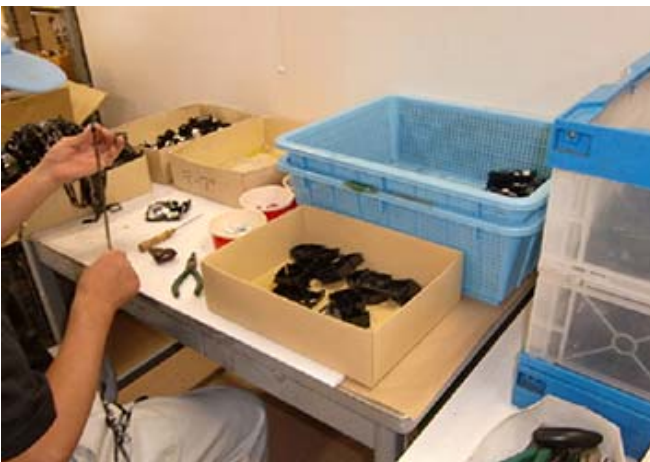
Disassembly and separation of tape cartridges and ink ribbon cassettes
