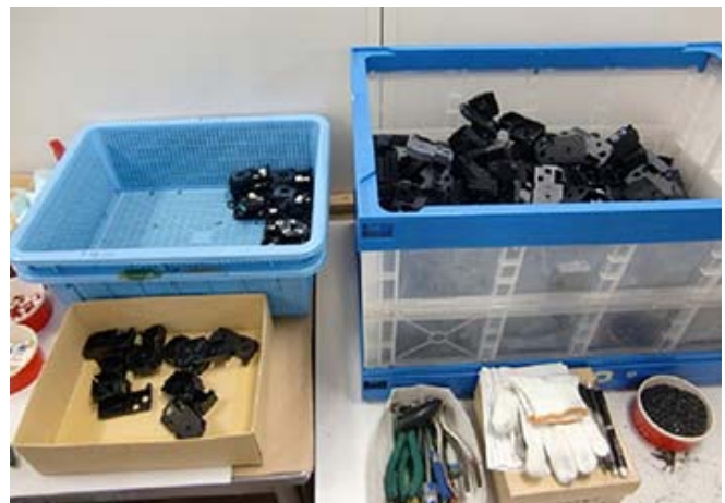
Disassembly and separation of tape cartridges and ink ribbon cassettes
