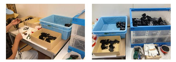
WorkDisassembly and separation of tape cartridges and ink ribbon cassettesshop (FY2020)
