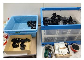
WorkDisassembly and separation of tape cartridges and ink ribbon cassettesshop (FY2020)
