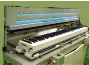
Automated sound quality tester on the piano keyboard production line
